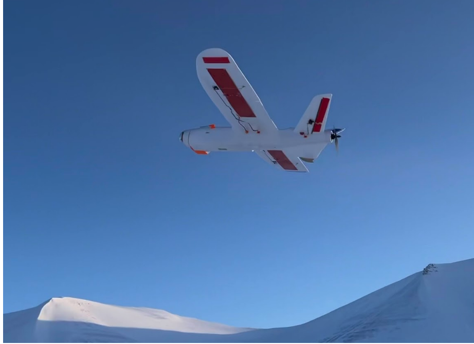
Figure 3.1: A Peregrine UAS in flight over the Slakbreen Glacier in Svalbard. Peregrine is a 2-meter wingspan fixed-wing UAS with an ice-penetrating radar instrument. The red radar antennas are visible under each wing.
